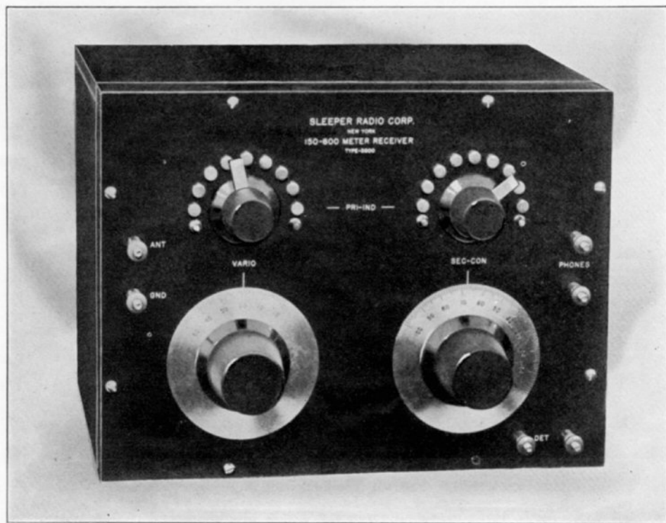
Fig. 1 A splendid receiving tuner for short wave reception. Units and ten switches control the primary inductances while a variable condenser tunes the secondary circuit
